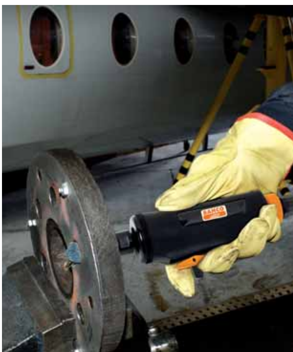
Thanks to the double collets included in the BP822, it can drive both 3 and 6 mm inserts
